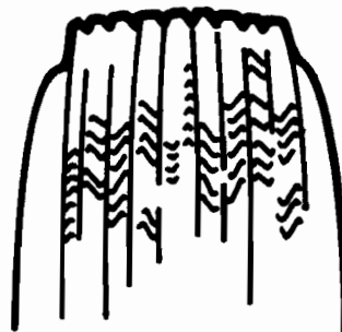
SAWTOOTH WEAR PATTERN DUE TO EXCESSIVE TOE-IN
